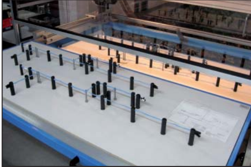
Harness board with a Fresenius cable harness.
