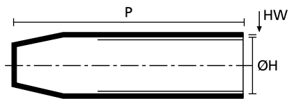
b: Fully recovered form (after heating)
