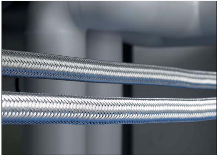
The HelaGuard PCSB galvanised steel conduit with a PVC coating galvanised steel overbraid offers high abrasion resistance and EMC screening.
