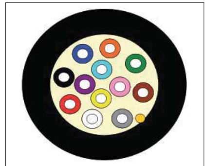
HellermannTyton's Tight Buffered Fibre Cable is available in OM4, OM3, OS1 and OS2
