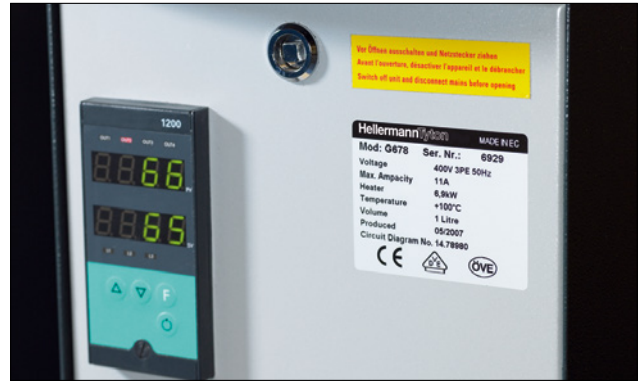
Professional type plate on a heating unit.
